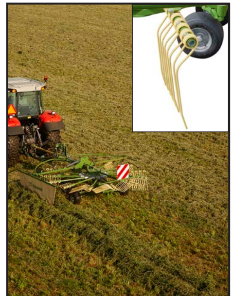
Above: Krone Lift Tines on the Swadro 42 T reduce contamination and create better windrows. Inset: New Krone Lift Tines are designed with angled ends.
