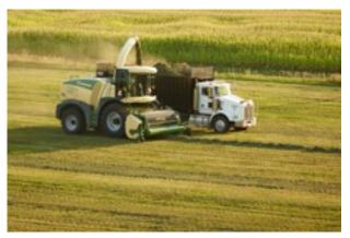
The exterior of the new models have been completely redesigned in order to increase visibility and function. The sloped body and low rear end allow the operator to easily see behind and to the side.
